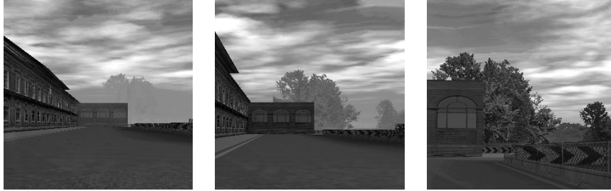
Figure 4: Fog is used to mask the popping up of trees in a game (eRacer ©Rage Software)
